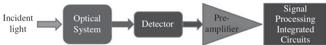
Simple schematic representation of a typical optical detector system
