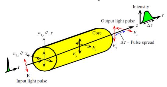
In optical fibers a phenomenon of birefringence can occur. The birefringence in fibers is described by a parameter called the mode birefringence  $B_m$ :
