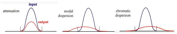
Dispersion, expressed in terms of the symbol  $\Delta t$ , is defined as pulse spreading in an optical fiber. As a pulse of light propagates through a fiber, elements such as numerical aperture, core diameter, refractive index profile, wavelength, and laser linewidth cause the pulse to broaden. This poses a limitation on the overall bandwidth of the fiber as demonstrated in Figure below (*Pulse broadening caused by dispersion*):
