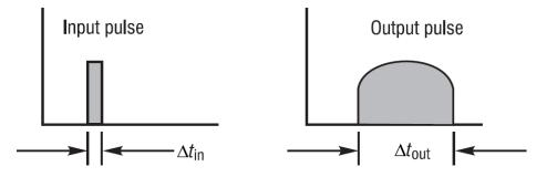
Dispersion  $\Delta t$  can be determined from Equation below:
