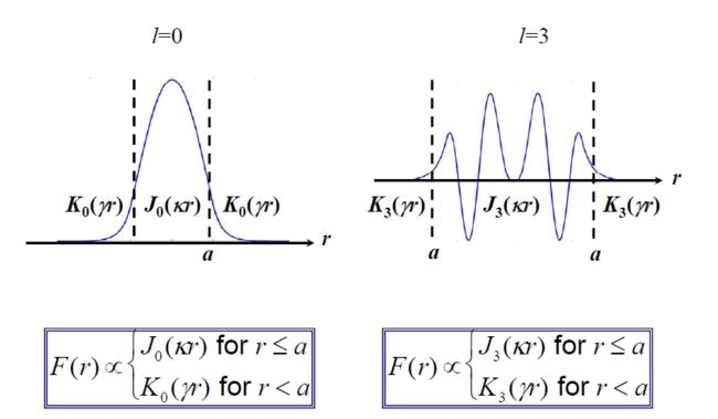
Boundary conditions at the core-cladding interface give a condition on the propagation constant  $\beta$  (characteristics equation)
