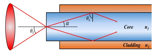
The *NA* is related to the critical angle  $\theta_c$  of the waveguide and it's defined as:
