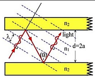
Propagation requires constructive interference
