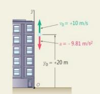
**a.** Velocity and Elevation. The *y* axis measuring the position coordinate (or elevation) is chosen with its origin *O* on the ground and its positive sense upward. The value of the acceleration and the initial values of *v* and *y* are as indicated. Substituting for *a* in a = dv/dt and noting that at t = 0,  $v_0 = +10$  m/s, we have
