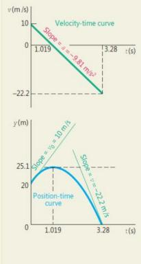
$\frac{dy}{dt} = v = 10 - 9.81t$   $\int_{y_0=20}^{y} dy = \int_{0}^{t} (10 - 9.81t) dt$   $[y]_{y_0}^{y} = [10t - 4.905t^2]_{0}^{t}$   $y - 20 = 10t - 4.905t^2$   $y = 20 + 10t - 4.905t^2 \quad (2)$
