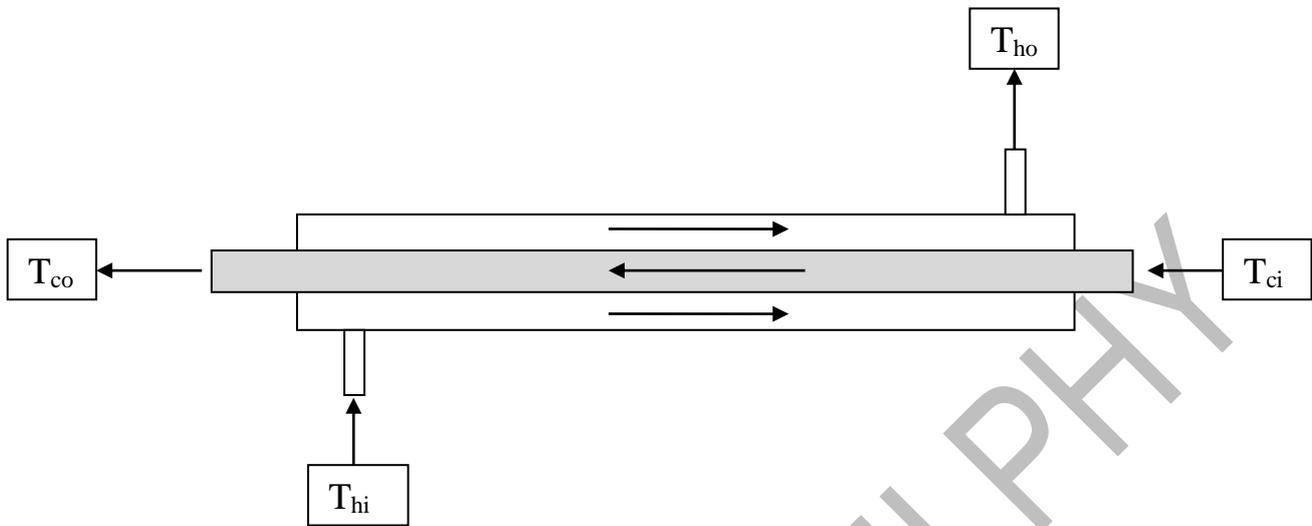
$$q_c = m_c C_{pc} (T_{co} - T_{ci})$$
