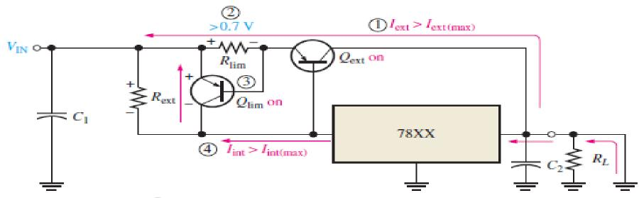
(b) When short occurs ①, the external current becomes excessive and the voltage across R<sub>lim</sub> increases ② and turns on Q<sub>lim</sub> ③, which then routes current through the regulator and conducts it away from Q<sub>ext</sub>, causing the internal regulator current to become excessive ④ which forces the regulator into thermal shut down.
