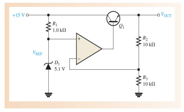
$V_{\text{REF}} = 5.1 \text{ V}$ , the zener voltage. The regulated output voltage is therefore  $V_{\text{OUT}} = \left(1 + \frac{R_2}{R_3}\right) V_{\text{REF}} = \left(1 + \frac{10 \text{ k}\Omega}{10 \text{ k}\Omega}\right) 5.1 \text{ V} = (2)5.1 \text{ V} = 10.2 \text{ V}$
