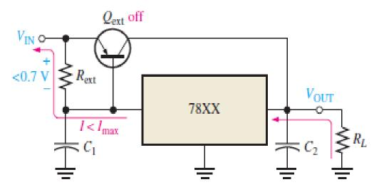
(a) When the regulator current is less than I<sub>max</sub>, the external pass transistor is off and the regulator is handling all of the current.
