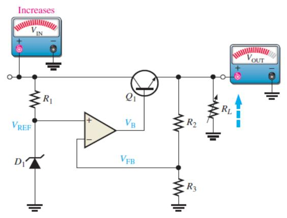
(b) When  $V_{\rm IN}$  or  $R_L$  increases,  $V_{\rm OUT}$  attempts to increase. The feedback voltage,  $V_{\rm FB}$ , also attempts to increase, and as a result,  $V_{\rm B}$ , applied to the base of the control transistor, attempts to decrease, thus compensating for the attempted increase in  $V_{\rm OUT}$  by decreasing the  $Q_1$  emitter voltage.
