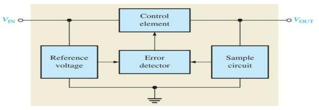
$\succ$  A basic op-amp series regulator is shown in Figure below:
