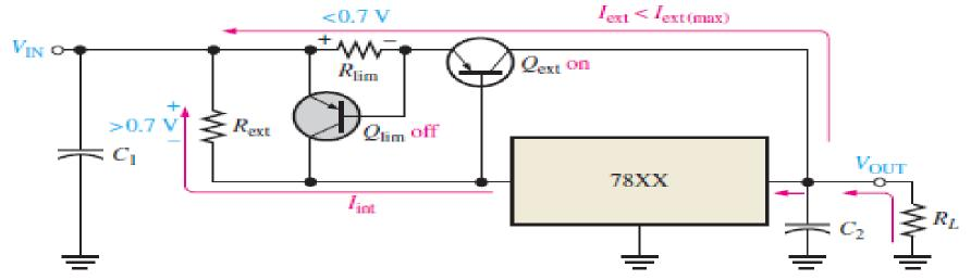
(a) During normal operation, when the load current is not excessive,  $Q_{\text{lim}}$  is off.
