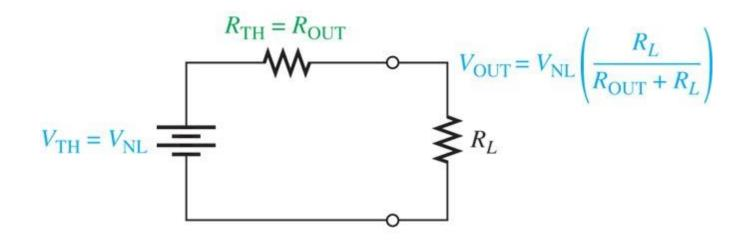
> R<sub>FL</sub> equal the smallest-rated load resistance, then V<sub>FL</sub>:
