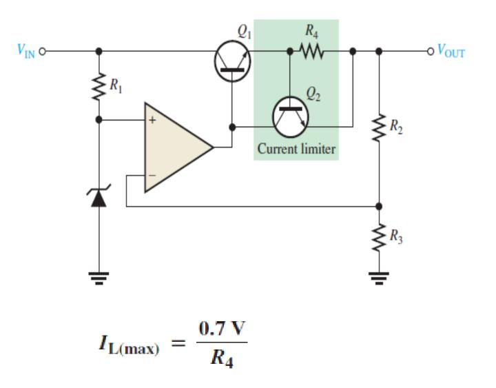
**Example 4.5:** Determine the maximum current that the regulator in figure below can provide to a load.
