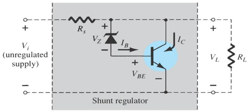
➢ Resistor R<sub>s</sub> drops the unregulated voltage depends on current supplied to load R<sub>L</sub>.
