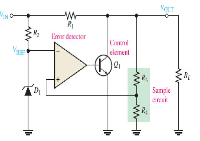
Sequence of responses when  $V_{OUT}$  tries to decrease as a result of a decrease in  $R_L$  or  $V_{IN}$  (opposite responses for an attempted increase).
