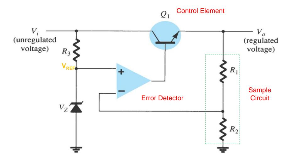
The resistor R<sub>1</sub> and R<sub>2</sub> sense a change in the output voltage and provide a feedback voltage.
