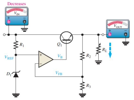
(a) When  $V_{\rm IN}$  or  $R_L$  decreases,  $V_{\rm OUT}$  attempts to decrease. The feedback voltage,  $V_{\rm FB}$ , also attempts to decrease, and as a result, the op-amp's output voltage  $V_{\rm B}$  attempts to increase, thus compensating for the attempted decrease in  $V_{\rm OUT}$  by increasing the  $Q_1$  emitter voltage. Changes in  $V_{\rm OUT}$  are exaggerated for illustration.
