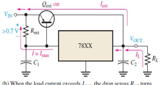
(b) When the load current exceeds I<sub>max</sub>, the drop across R<sub>ext</sub> turns Q<sub>ext</sub> on and it conducts the excess current.
