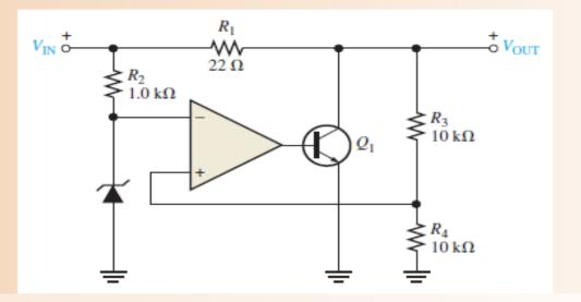
The worst-case power dissipation in  $R_1$  occurs when the output is short-circuited and  $V_{OUT} = 0$ . When  $V_{IN} = 12.5$  V, the voltage dropped across  $R_1$  is
