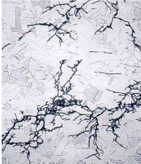
SCC in a 316 stainless steel chemical processing piping system; photo courtesy
