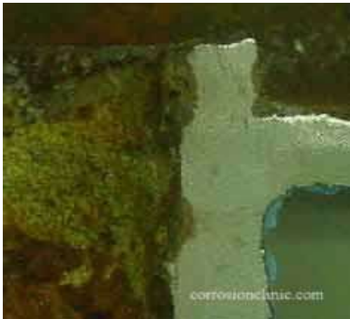
Graphitic corrosion of a gray cast iron valve
