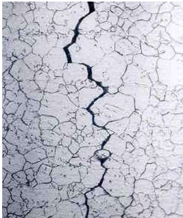
intergranular SCC of an Inconel heat exchanger tube with the crack following the grain boundaries
