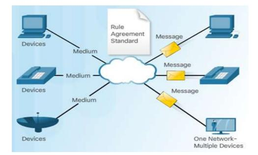
Today, the separate data, telephone, and video networks are converging. Unlike dedicated networks, converged networks are capable of delivering data, voice, and video between many different types of devices over the same network infrastructure, as shown in the figure. This network infrastructure uses the same set of rules, agreements, and implementation standards
