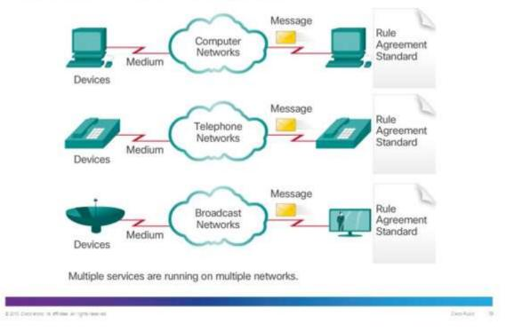
Consider a school built thirty years ago. Back then, some classrooms were cabled for the data network, telephone network, and video network for televisions. These separate networks could not communicate with each other, as shown in the figure. Each network used different technologies to carry the communication signal. Each network had its own set of rules and standards to ensure successful communication.
