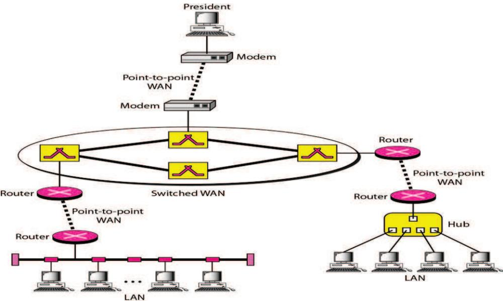
*Fig. (1.12): A heterogeneous network made of four WANs and two LANs.*
