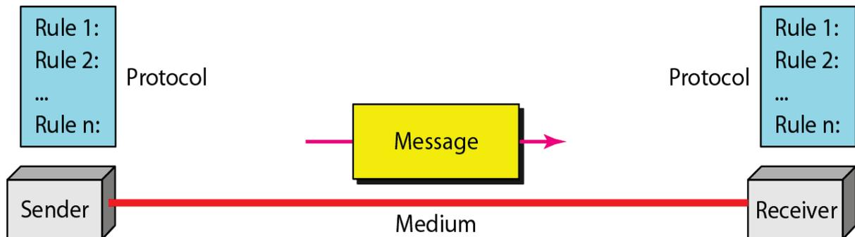
*Fig. (1.1): Five components of data communication system.*
