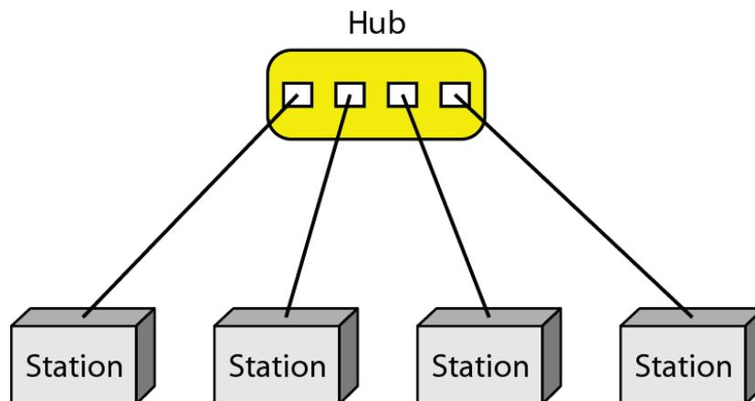
*Fig. (1.6): A star topology connecting four stations*
