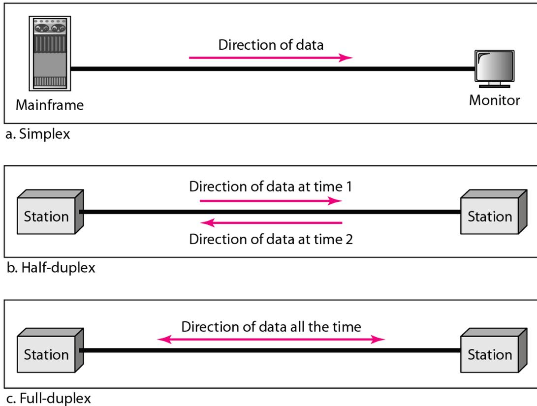
*Fig. (1.2): Data flow (simplex, half-duplex and full-duplex).*
