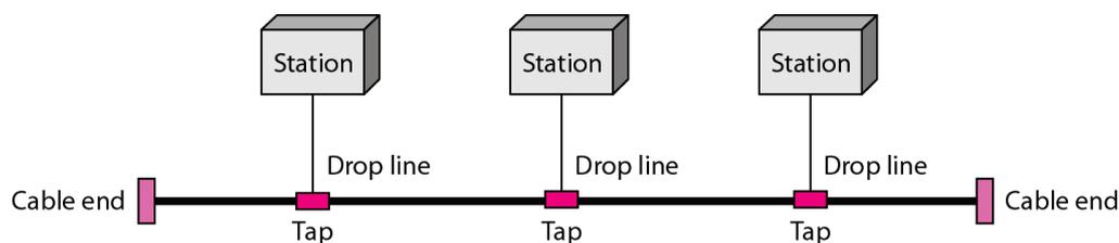
*Fig. (1.7): A bus topology connecting three stations.*
