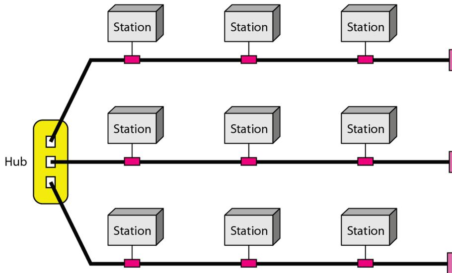
*Fig. (1.9): A hybrid topology: a star backbone with three bus networks.*
