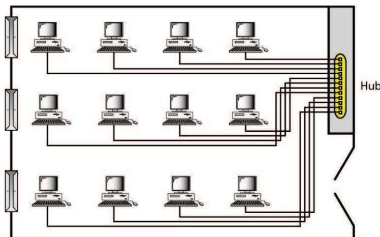
*Fig. (1.10): An isolated LAN connecting 12 computers to a hub in a closet*
