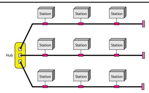
Fig. (1.9): A hybrid topology: a star backbone with three bus networks.
