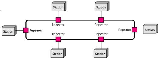
Fig. (1.8): A ring topology connecting six stations.
