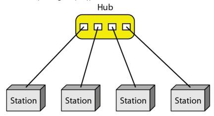
Fig. (1.6): A star topology connecting four stations
