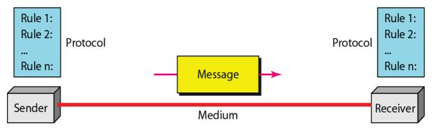
Fig. (1.1): Five components of data communication system.
