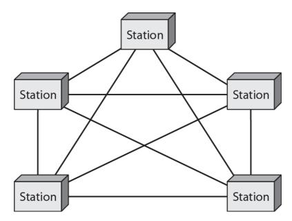
Fig. (1.5): A fully connected mesh topology (five devices)
