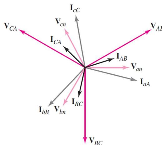
Fig. 4.13: A phasor diagram that could apply to the circuit of Fig. 4.12 if  $Z_p$  were an inductive impedance.
