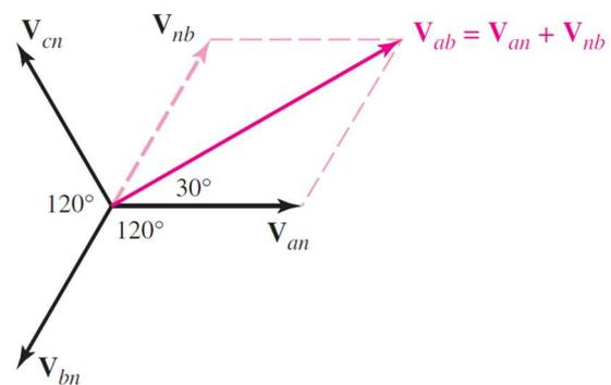
Fig. 4.2 The phasor diagram
