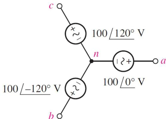
Fig. 4.1 Three phase power supply.
