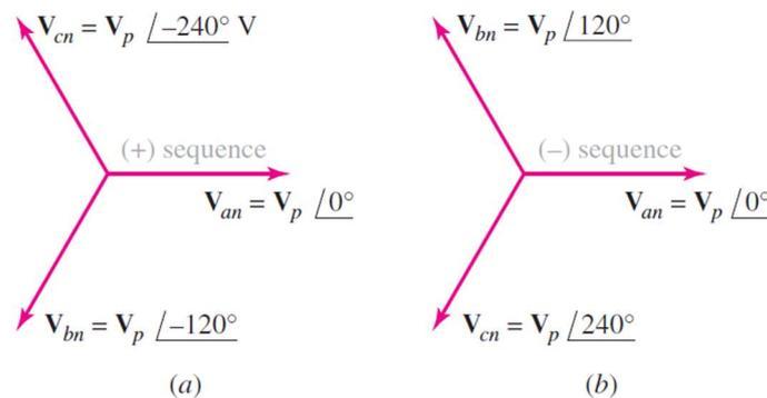
Fig. 4.7: (a) Positive, or abc, phase sequence. (b) Negative, or cba, phase sequence.
