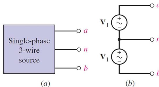
Fig. 4.3 (a) A single-phase three-wire source. (b) The representation of a single-phase three-wire source by two identical voltage sources.
