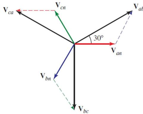
Fig. 4.8: A phasor diagram which is used to determine the line voltages from the given phase voltages. Or, algebraically,  $V_{ab} = V_{an} - V_{bn} = V_p \angle 0^\circ - V_p \angle -120^\circ = V_p - V_p \cos(-120^\circ) - jV_p \sin(-120^\circ) = V_p(1 + 1/2 + j\sqrt{3}/2) = \sqrt{3}V_p \angle 30^\circ$ .
