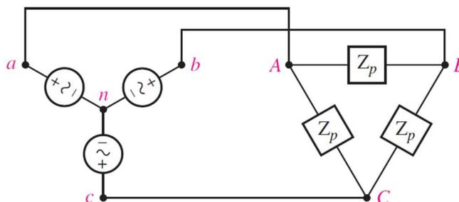
Fig. 4.12: A balanced Δ-connected load is present on a three-wire three-phase system. The source happens to be Y-connected.
