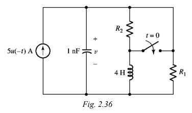
We note that at  $t = 0^-$ , the current source is on, and the inductor can be treated as a short circuit. Thus,  $v(0^-)$  appears across  $R_2$ , and is given by  $v(0^-) = 5R_2$  and a value of 400 m $\Omega$  should be selected for  $R_2$  to obtain v(0) = 2 V.
