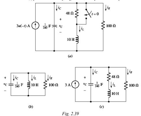
At t=0, both the 3 A source and the 48  $\Omega$  resistor are removed, leaving the circuit shown in Fig. 3.39b. Thus,  $\alpha=1.2~{\rm s}^{-1}$  and  $\omega_0=4.899~{\rm rad/s}$ . Since  $\alpha<\omega_0$ , the circuit is underdamped, and we therefore expect a response of the form
