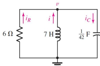
We will select R, increasing its value until critical damping is obtained, and thus leave  $\omega_0$  unchanged. The necessary value of R is  $7\sqrt{6}/2 \Omega$ ; L is still 7 H, and C remains 1/42 F. We thus find
