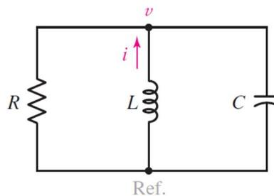
*Fig. 2.28: The source-free parallel RLC circuit.*
