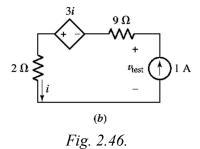
As we are interested only in  $v_C(t)$ , it is perfectly acceptable to begin by finding the Thévenin equivalent resistance connected in series with the inductor and capacitor at  $t = 0^+$ . We do this by connecting a 1 A source as shown in Fig. 2.46b, from which we deduce that
