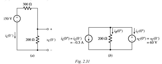
In Fig. 2.31b, we draw the circuit at  $t = 0^+$ , representing the inductor current and capacitor voltage by ideal sources for simplicity. Since neither can change in zero time, we know that  $v_C(0^+) = 60 \text{ V}$ . We have an equation for the capacitor voltage:
