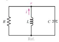
Fig. 2.28: The source-free parallel RLC circuit.
