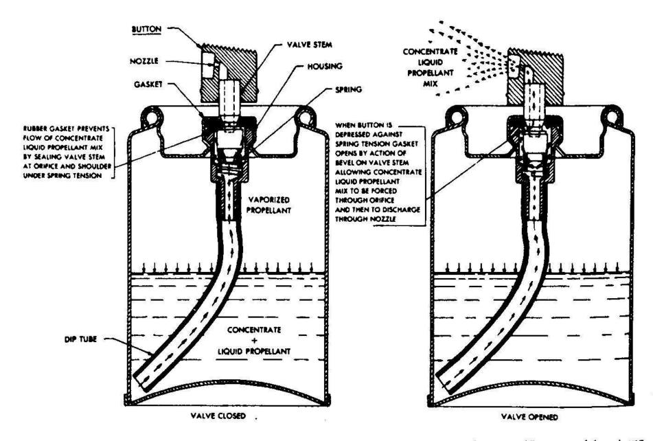
Fig. 13-2. Cross section sketches of contents and operation of a typical two-phase aerosol system. (Courtesy of Armstrong Laboratories, Inc., Division of Aerosol Techniques, Inc.)
