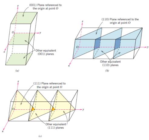
Representations of a series each of (a) (001), (b) (110), and (c) (111) crystallographic planes Construct a  $(0\overline{1}1)$  plane within a cubic unit cell.
