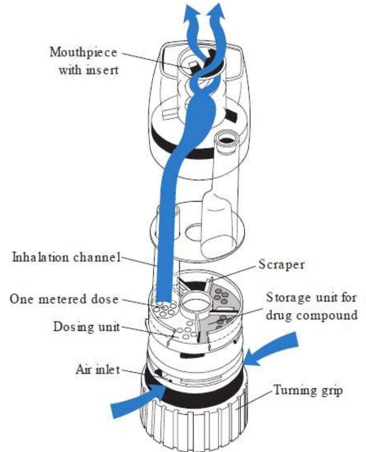
Fig. 37.8 • The Turbohaler®. (Courtesy of AstraZeneca.)
