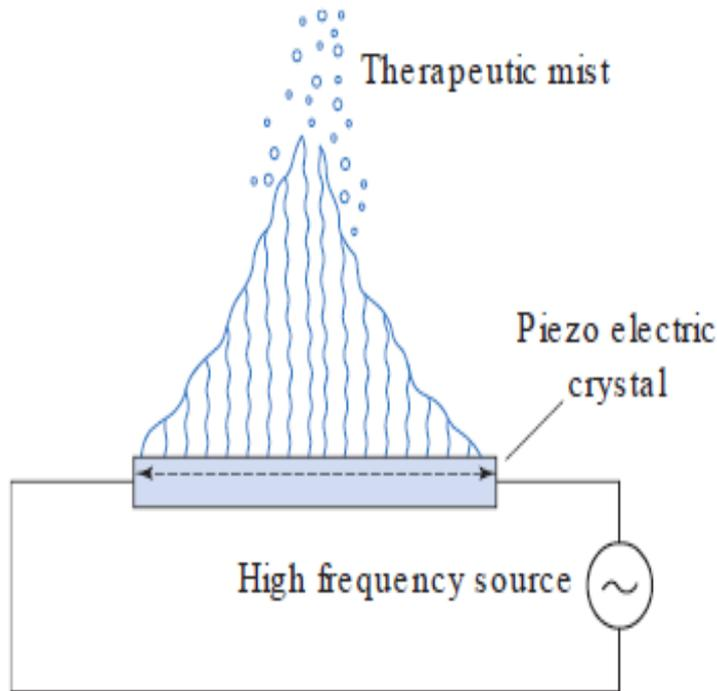
Fig. 37.11 • Schematic diagram of an ultrasonic nebulizer. (Courtesy of Atkins et al, 1992, with permission.)
