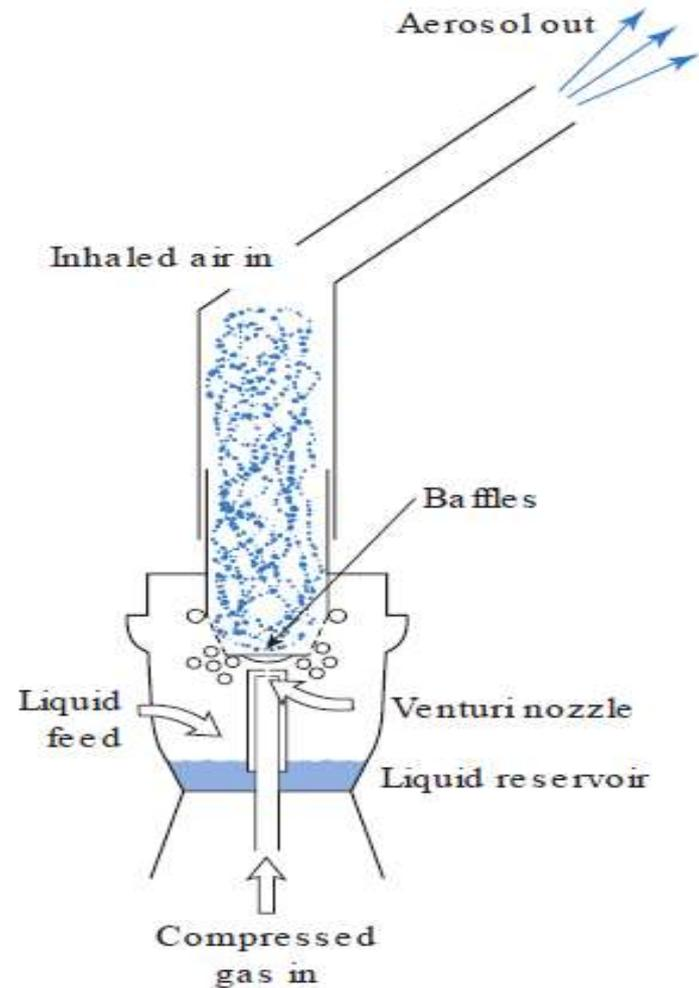
Fig. 37.10 • Schematic diagram of a jet nebulizer. Compressed gas passes through a Venturi nozzle, where an area of negative pressure is created. Liquid is drawn up a feed tube and is fragmented into droplets. Large droplets impact on baffles, and small droplets are carried away in the inhaled air stream.
