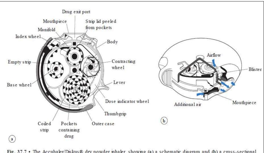
Fig. 37.7 • The Accuhaler/Diskus® dry powder inhaler, showing (a) a schematic diagram and (b) a cross-sectional representation of the device. (Courtesy of Prime et al, 1996, with permission.)
