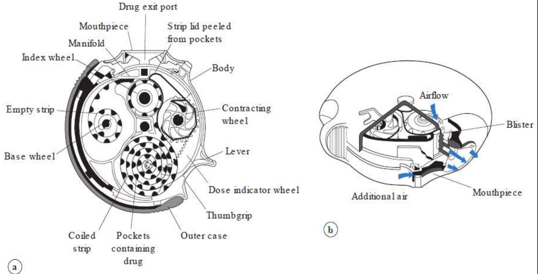
Fig. 37.7 • The Accuhaler/Diskus® dry powder inhaler, showing (a) a schematic diagram and (b) a cross-sectional representation of the device. (Courtesy of Prime et al, 1996, with permission.)
