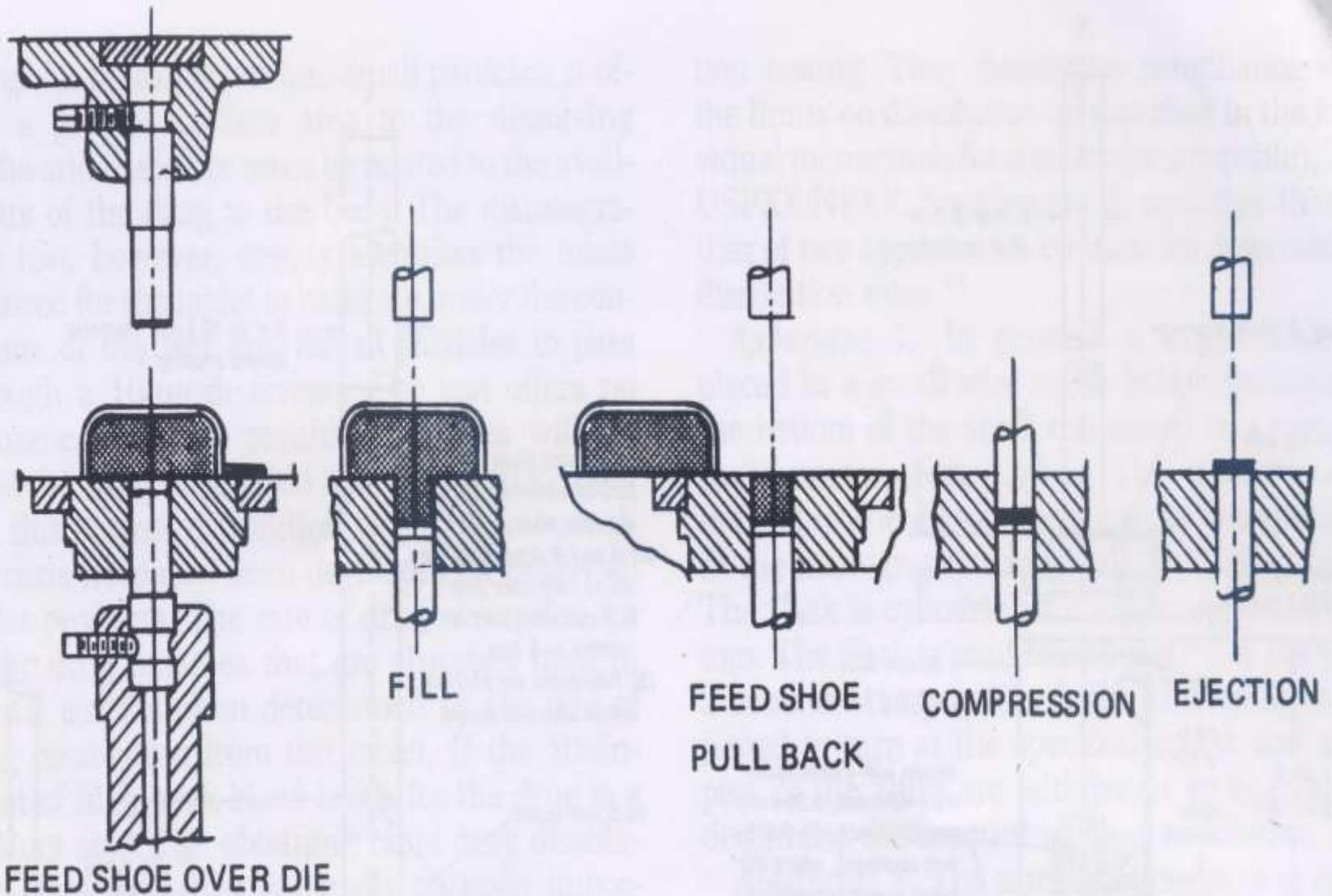
FIG. 11-5. The compression cycle of a single-punch tablet press. (Courtesy of Vector Corporation, Marion, IA.)
