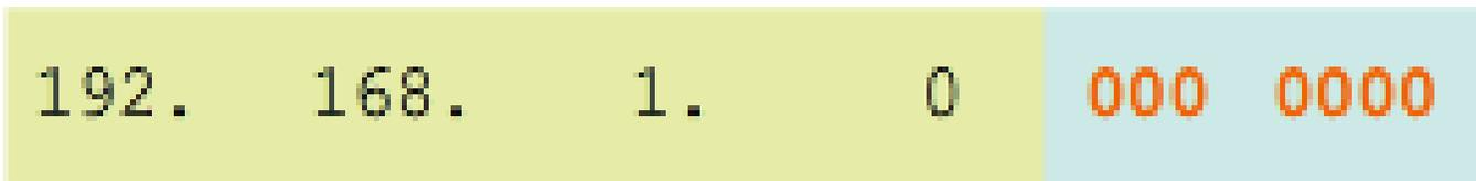
The diagram shows a 32-bit IP address: 192.168.1.00000000. The first four octets (192.168.1.0) are highlighted in a light green background, representing the network prefix. The last two octets (00000000) are highlighted in a light blue background, representing the host field. An orange arrow points from a box below to the host field.
