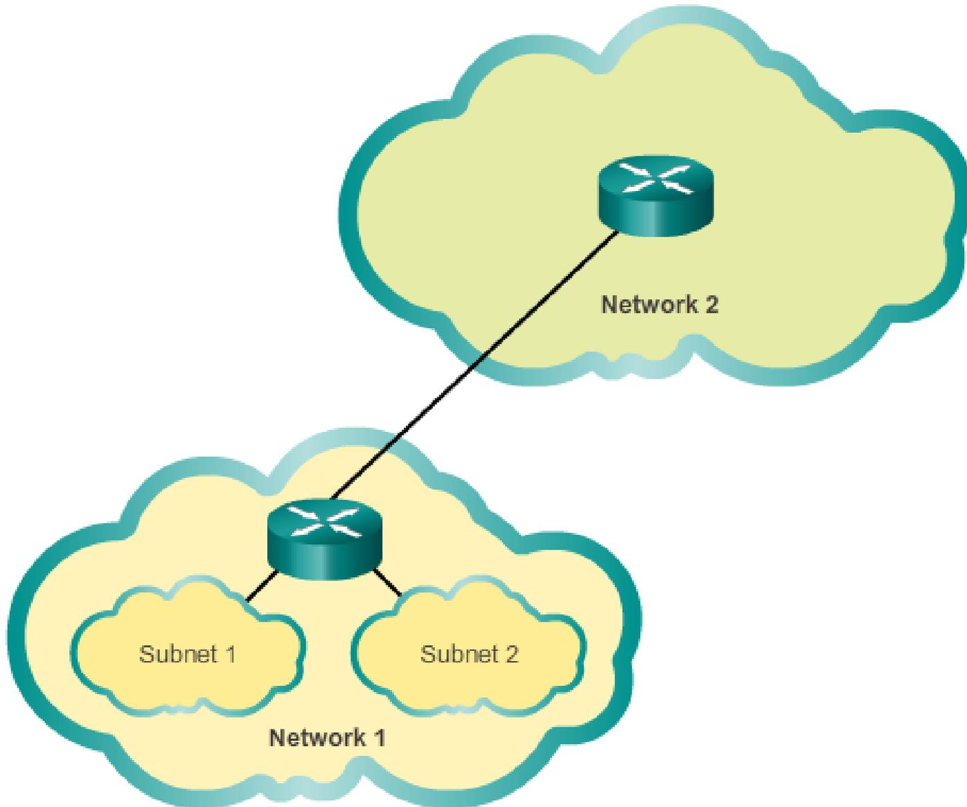
A router is necessary for devices on different networks to communicate. Devices on a network use the router interface attached to their LAN as their default gateway. Traffic that is destined for a device on a remote network will be processed by the router and forwarded toward the destination. To determine if traffic is local or remote, the router uses the subnet mask.
