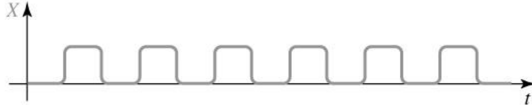
(b) Oscillation at inverter output
