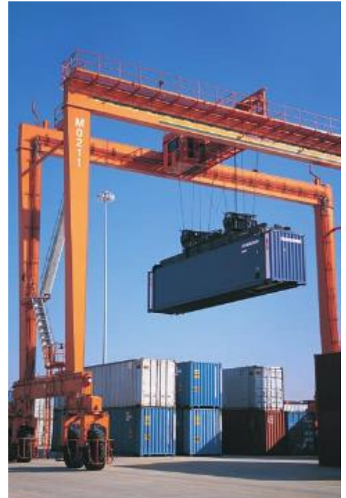
Photo 11.2 Multiple cables and pulleys are used by this shipyard crane.
