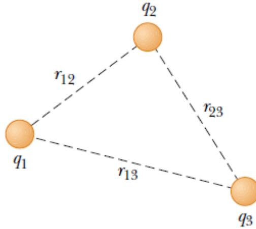
$$U = k_e \left( \frac{q_1 q_2}{r_{12}} + \frac{q_1 q_3}{r_{13}} + \frac{q_2 q_3}{r_{23}} \right)$$
