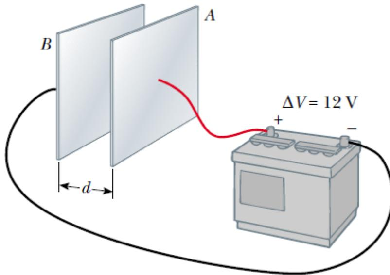
$$E = \frac{|V_B - V_A|}{d} = \frac{12 \text{ V}}{0.30 \times 10^{-2} \text{ m}} = 4.0 \times 10^3 \text{ V/m}$$
