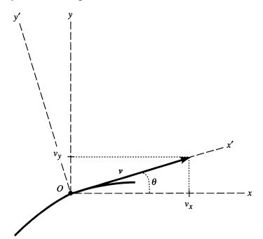
**Figure 1.8.2** Velocity of a moving particle referred to two different two-dimensional coordinate systems.
