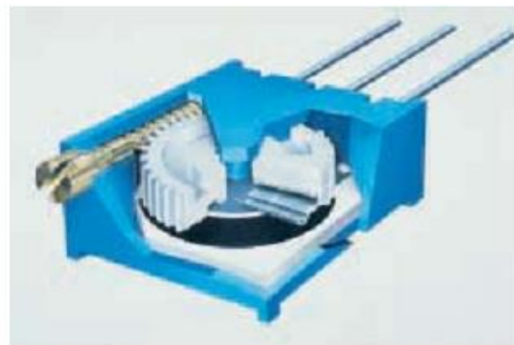
(b) Internal view of variable resistor.
