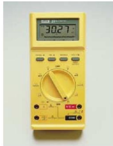
(b) Hand-held digital multimeter (DMM). (Reproduced with permission from the John Fluke Mfg. Co., Inc.)
