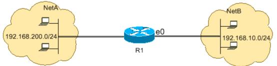
This configuration allows the IP packets with an IP header that has a source address in the network 192.168.10.0/24 and a destination address in the network 192.168.200.0/24 access to NetA. There is the implicit deny all clause at the end of the ACL which denies all other traffic passage through Ethernet 0 inbound on R1.
