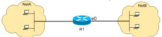
Telnet uses TCP, port 23. This configuration shows that all TCP traffic destined to NetA for port 23 is blocked, and all other IP traffic is permitted.
