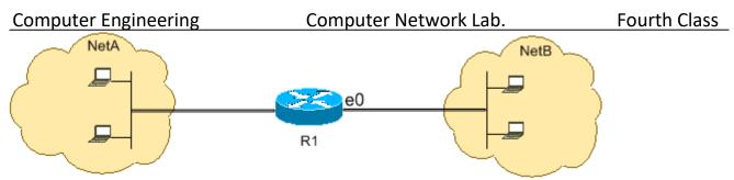
This configuration permits only echo-reply (ping response) packets to come in on interface Ethernet 0 from NetB towards NetA. However, the configuration blocks all echo-request ICMP packets when pings are sourced in NetB and destined to NetA. Therefore, hosts in NetA can ping hosts in NetB, but hosts in NetB cannot ping hosts in NetA.
