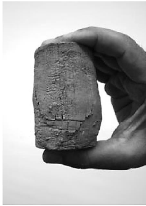
Figure (12.30) Failure by bulging of an unconfined compression test specimen
