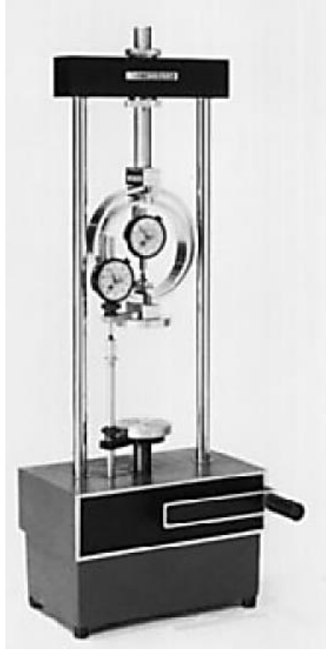
Figure 12.28 Unconfined compression test equipment
