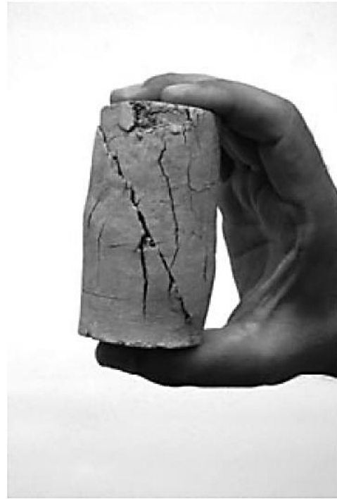
Figure 12.29 Failure by shear of an unconfined compression test specimen
