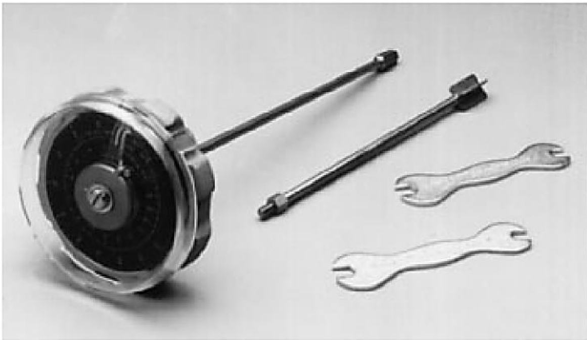
Figure 12.33 Laboratory vane shear test device (Courtesy of ELE International)
