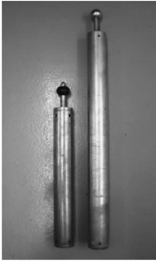
Figure (6.6) Comparison between standard Proctor hammer (left) and modified Proctor hammer (right)
