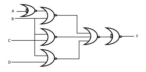
**Ex.** : Using NAND Gate only and NOR Gate only to simplify the following function:  $F = \sum_{(0,1,2,5,8,9,10,13)}$
