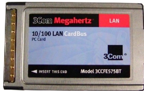
Uses CardBus; is 54 mm wide by 85.6 mm long
