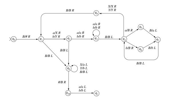
Processing the null string uses the arc from  $q_1$  to  $q_f$ . Shifting a string one square to the right is accomplished by states  $q_3$  to  $q_7$ . The arc from  $q_4$  to  $q_8$  when the shift has been completed. If another shift is needed, the entire process is repeated by entering  $q_1$ .
