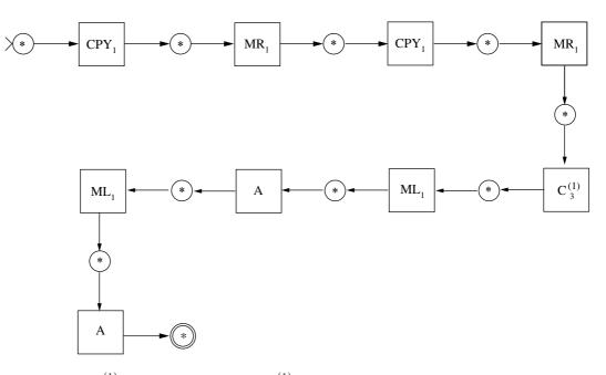
The machine  $C_3^{(1)}$  computes the function  $c_3^{(1)}$ , which was shown to be Turing computable in Example 9.4.2. Tracing the computation of M with input *n* illustrates the interaction among the machines that make up M.
