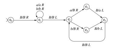
On reading the first blank following the input, the head moves to the left. If the input is the null string, the computation halts in state  $q_f$  with the tape head in position zero as desired. Otherwise, an a is moved to the right by transitions to states  $q_2$  and  $q_3$ . Similarly, states  $q_4$  and  $q_3$  shift a b. This process is repeated until the entire string has been shifted.
