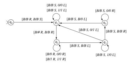
The cycle of producing and writing a string on tape 1 begins in  $q_1$ . A # is written on tape 1 followed by the string in the input position on tape 2. For the remainder of the cycle, the tape head on tape 1 remains stationary while the next string is generated on tape 2.
