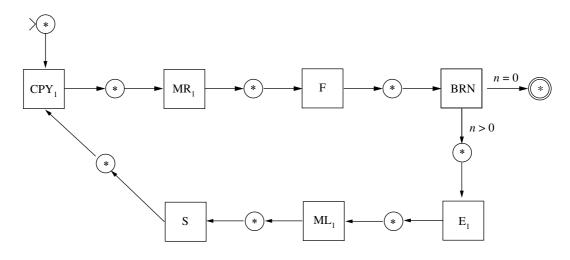
The computation begins with the counter  $\overline{0}$  on the tape. A working copy of  $\overline{0}$  is made and F is run on the copy. The BRN macro is used to determine whether the computed value of f is 0. If not, the computed value is erased, the counter is incremented, and the subsequent f value is computed. The cycle of generating a natural number and computing the f value halts when a natural number n is found for which f(n) = 0.
