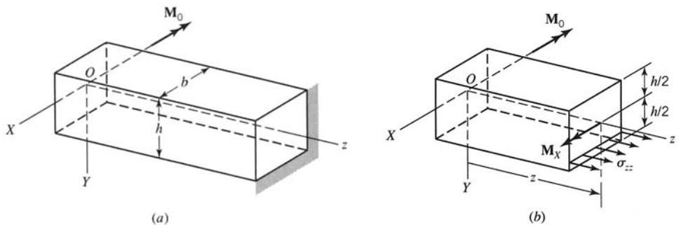
FIGURE 7.5 Cantilever beam with rectangular cross section.
