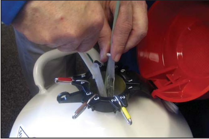
When all straws are used in the top goblet, remove and discard it.
