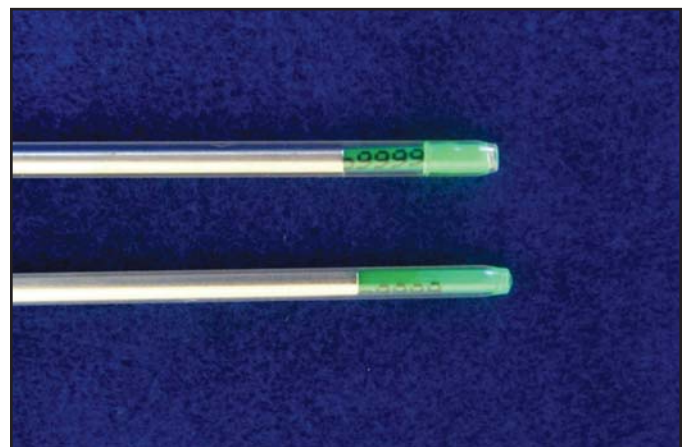
Proper seal between straw and sheath is extremely important.
