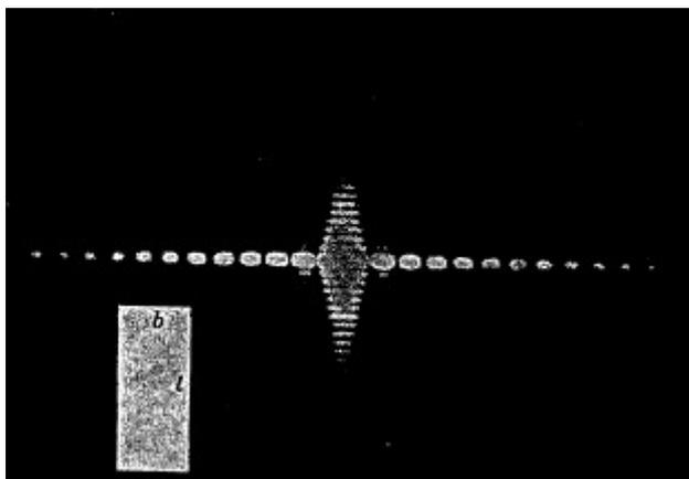
Figure 15G Diffraction pattern from a rectangular opening.
