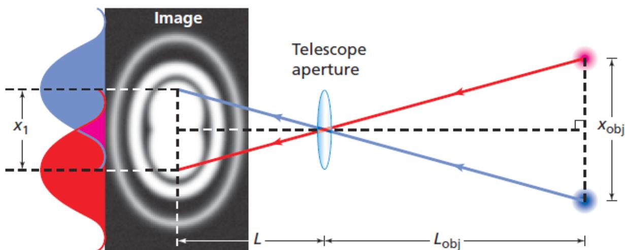
**Figure 1.** Similar-triangle geometry allows you to calculate the actual separation distance of objects. The blue and red colors are used only for the purpose of illustration
