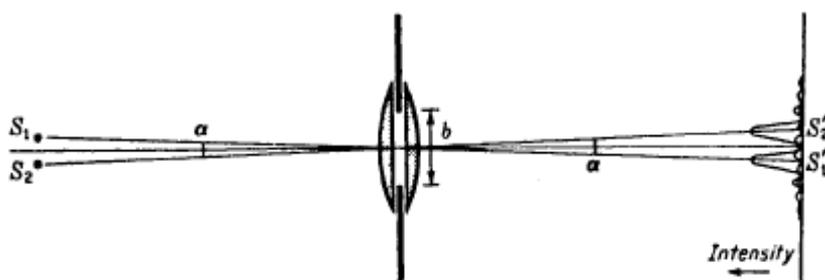
Figure 15H Diffraction images of two slit sources formed by a rectangular aperture.
