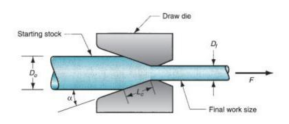
Figure 9.1 Drawing of bar, rod, or wire.
