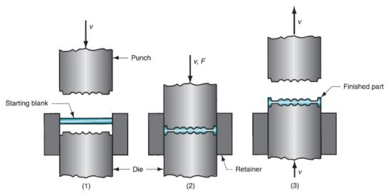
Figure 7.10 Coining operation: (1) start of cycle, (2) compression stroke, and (3) ejection of finished part.
