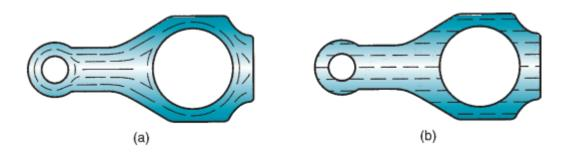
Figure 7.7 Comparison of metal grain flow in a part that is: (a) hot forged with finish machining, and (b) machined complete.
