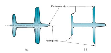
Figure 7.8 Cross sections of (a) conventional-and (b) precision forgings. Dashed lines in (a) indicate subsequent machining required to make the conventional forging equivalent in geometry to the precision forging. In both cases, flash extensions must be trimmed.
