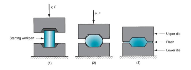
Figure 7.6 Sequence in impression-die forging: (1) just prior to initial contact with raw workpiece, (2) partial compression, and (3) final die closure, causing flash to form in gap between die plates.
