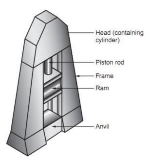
Figure 7.11 Diagram showing details of a drop hammer for impression-die forging.
