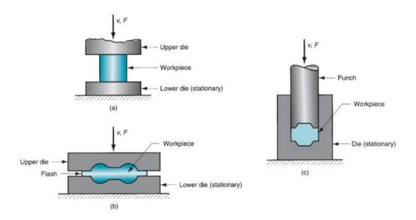
Figure 7.1 Three types of forging operation illustrated by cross-sectional sketches:
