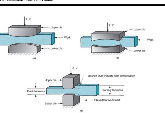
Figure 7.5 Several open-die forging operations:
