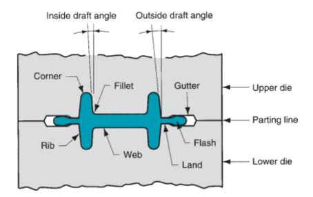
Figure 7.12 Terminology for a conventional impression-die in forging.
