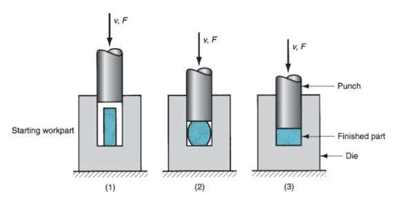
Figure 7.9 Flashless forging: (1) just before initial contact with workpiece, (2) partial compression, and (3) final punch and die closure. Symbols v and F indicate motion (v = velocity) and applied force, respectively.
