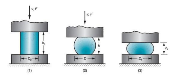
Figure 7.3 Actual deformation of a cylindrical workpart in open-die forging, showing pronounced barreling: (1) start of process, (2) partial deformation, and (3) final shape.
