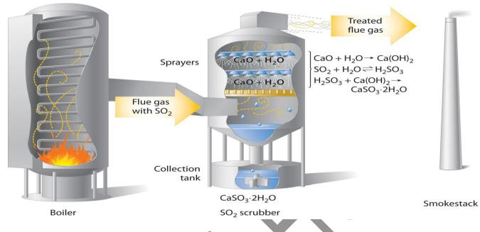
Fig(1): Schematic Diagram of a Wet Scrubber System.
