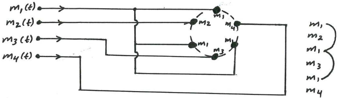
b) The commutator speed in (sample/sec.) represents the total sampling frequency of the TDM system.
