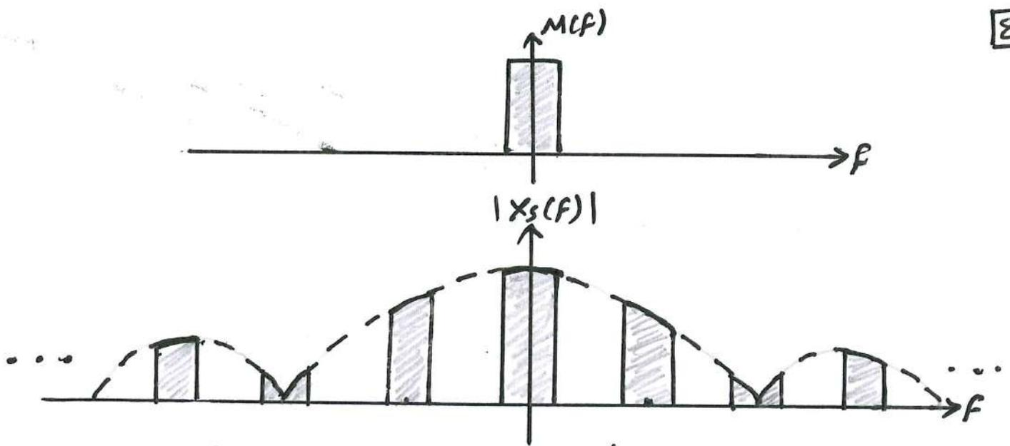
\* The signal can be reconstructed by a (LPF) but the resulted signal is not exactly the same as the original one because of the frequency domain distortion caused by the sinc function.
