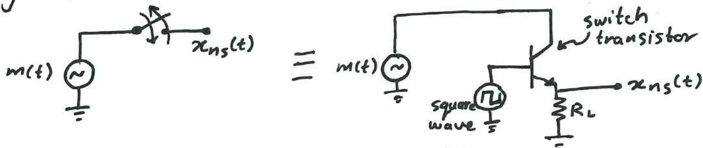
The above circuit can be modeled theoretically by multiplying  $m(t)$  by a train of gate function or (rectangular pulses) called  $x_p(t)$ .
