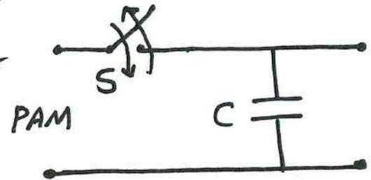
pulse. Therefore, the capacitor (C) is charged up to the pulse amplitude when (S) is closed, and it holds this value when (S) is opened during the interval between two pulses. As a result, the detected signals are as shown below:
