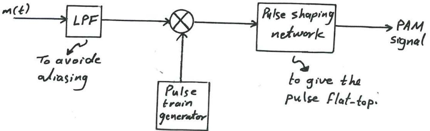
The above block diagram gives the details of PAM modulation. However, it can simply be generated using the (S/H) circuit explained previously.
