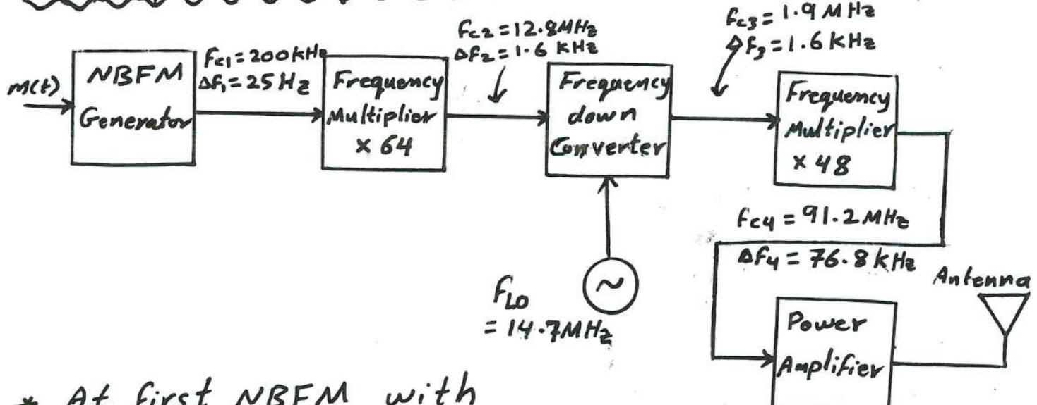
\* At first NBFM with  $f_{c1} = 200\text{ kHz}$  and  $\Delta f_1 = 25\text{ Hz}$  is generated
