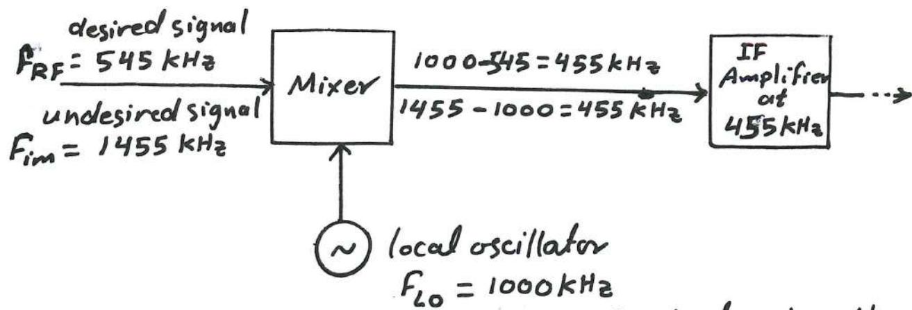
Local oscillator frequency is adjusted using the following equation :
