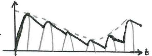
\* During the +ve half cycle of the carrier, the diode (D) is forward biased and (C) charged up to the peak value of the carrier. As the signal falls below the max. value, the capacitor (C) slowly discharge through the resistance (R) until the next +ve half-cycle.
