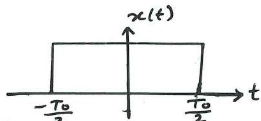
This signal has a finite duration, so it can be an energy signal if  $0 < E < \infty$ . Therefore, let's check its energy:
