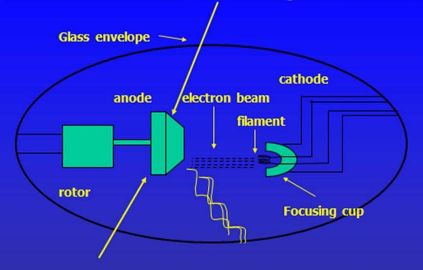
The anode is usually composed of tungsten or molybdenum as it must withstand very high temperatures (>3000 degrees C)
