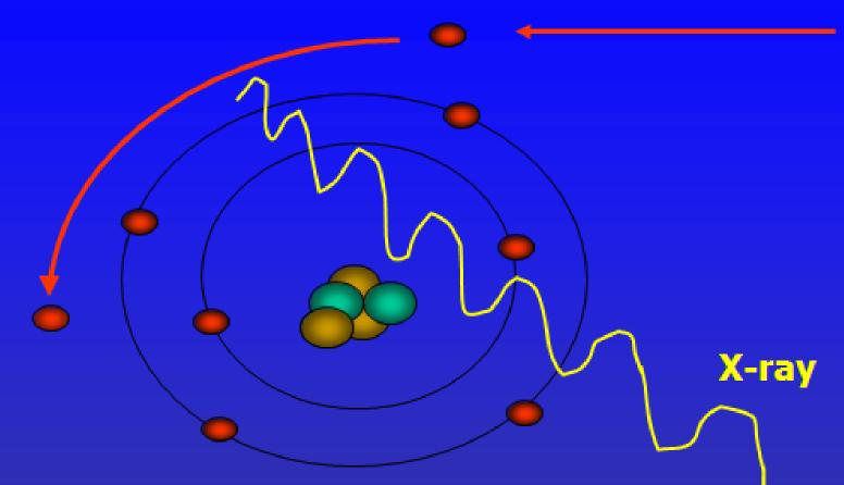
Projectile electrons originating from the cathode filament impinge on atoms in the anode and will often pass close by the nucleus of these atoms.
