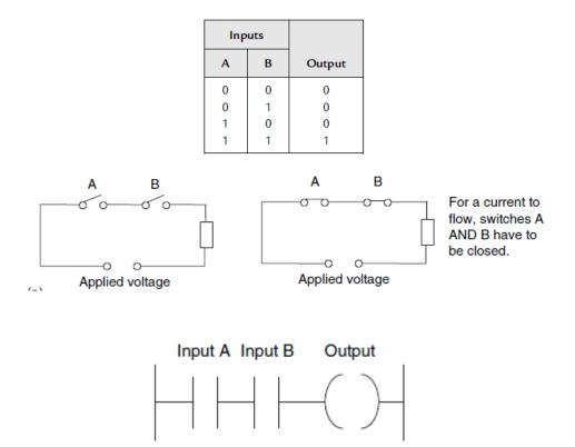
On a ladder diagram, contacts in the horizontal rung or in series, represent the logical AND operation.
