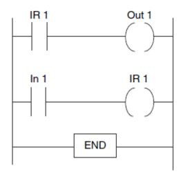
IR 1 not energized as a result of input to In 1 in the first scan until the second scan of the program.
