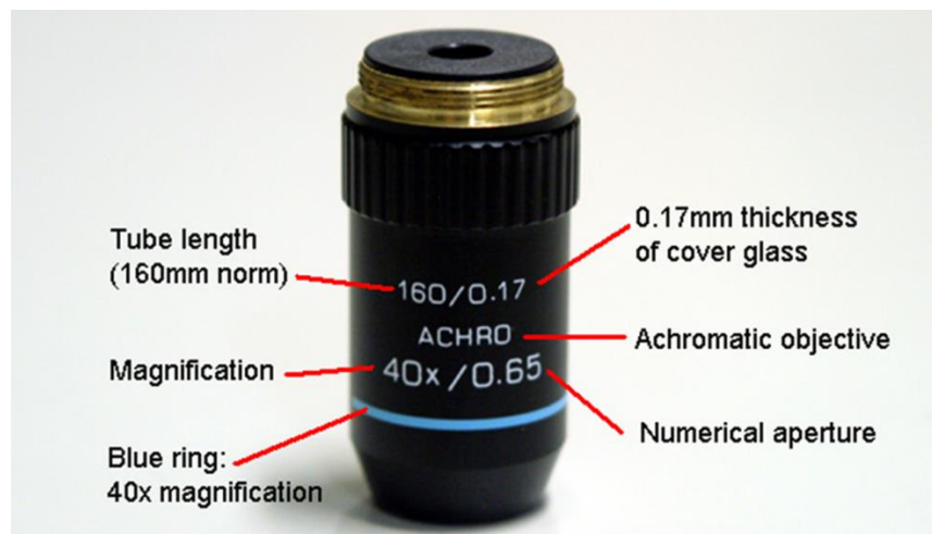
Figure 2.6 the parameters of microscope objectives
