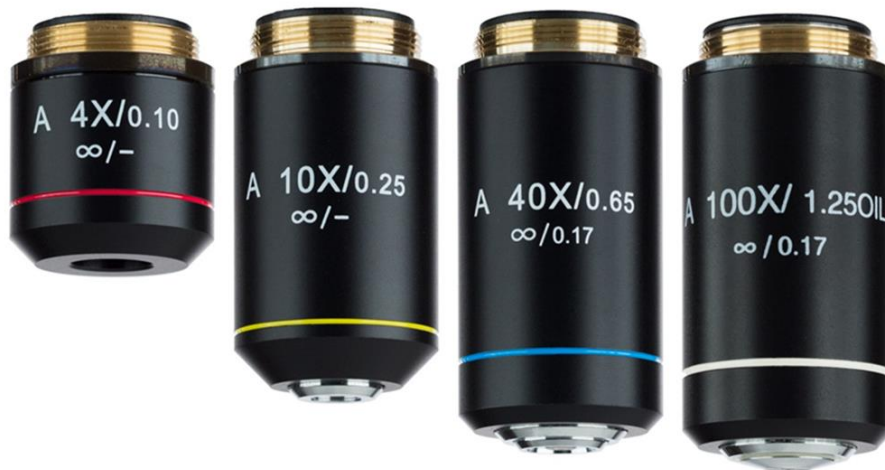
Figure 2.5 the color coding bands of microscope objectives
