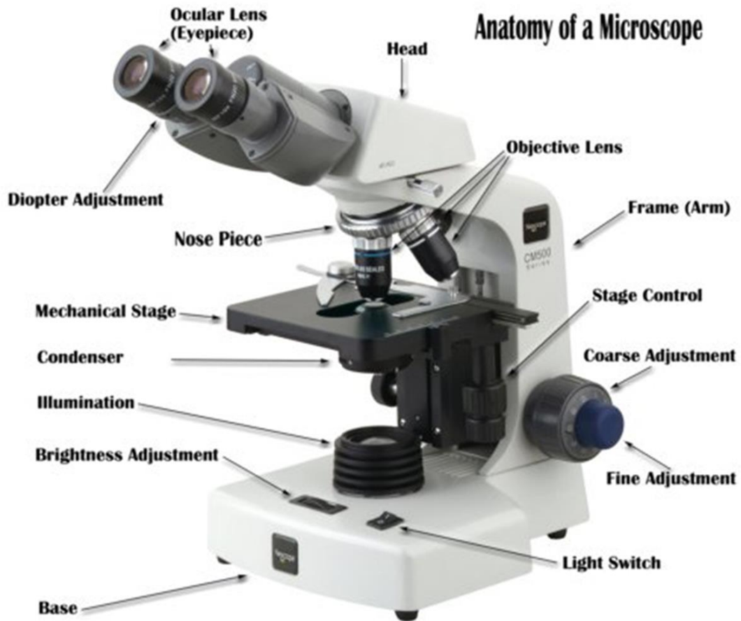
Figure 2.9 represent all parts of the light compound microscope
