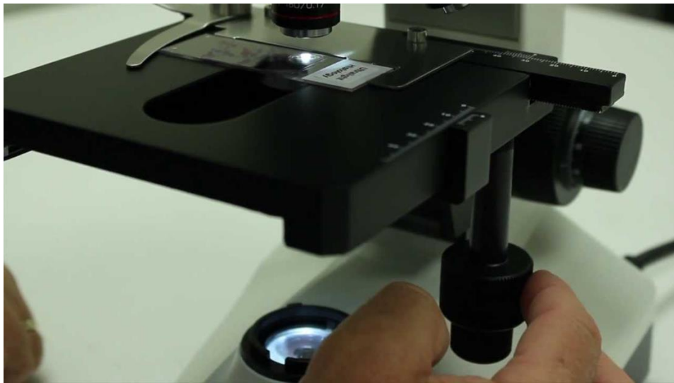
Figure 2.8 Movable stage of the microscope
