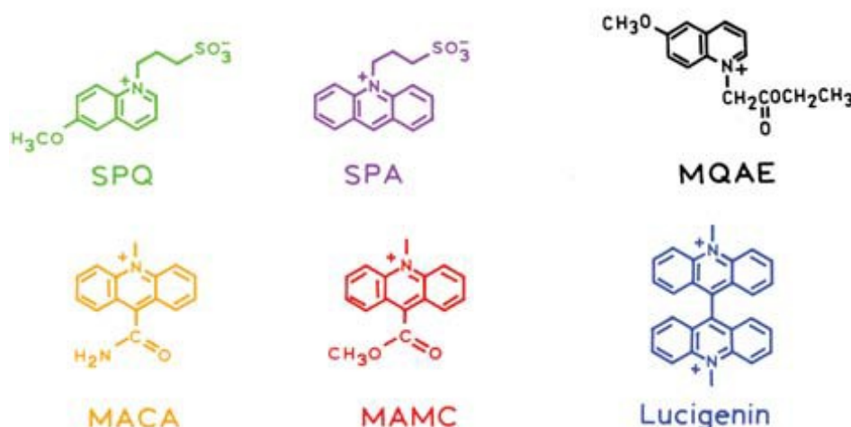
Figure 5. Representative chloride probes. These probes are collisionally quenched by chloride
