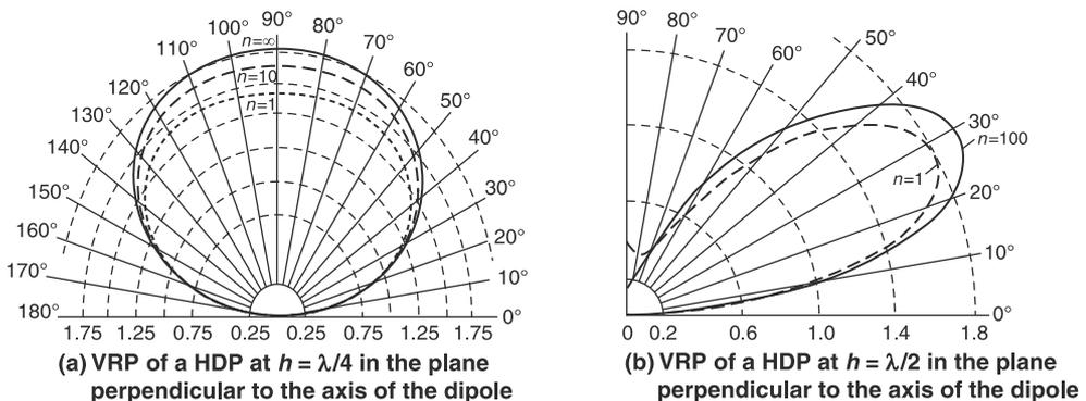
**Figure 2-10** Vertical radiation pattern of horizontal dipole at  $h = \lambda/4$  and  $h = \lambda/2$ .
