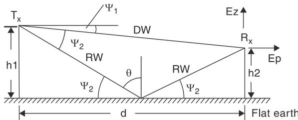
**Figure 2-2** Direct wave (DW) and reflected wave (RW) between  $T_x$  and  $R_x$ .
