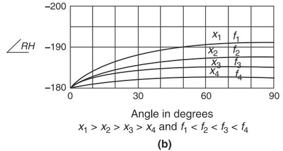
**Figure 2-3** Variation of  $|R_h|$  and  $\angle R_h$  with incident angle.
