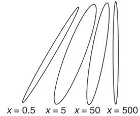
**Figure 2-7** Elliptical polarization and tilt of  $E$  at the earth surface for  $\epsilon_r = 5$  and for different values of  $x$ .
