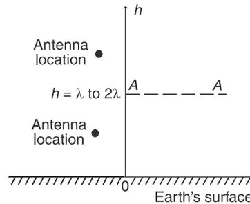
**Figure 2-6** Transition between surface and space waves.
