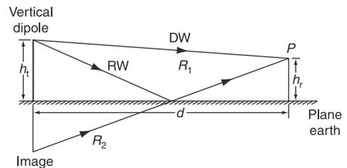
**Figure 2-5** Vertical dipole and its image.
