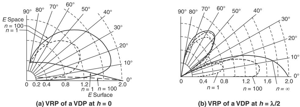
**Figure 2-9** Vertical radiation pattern of vertical dipole at  $h = 0$  and  $h = \lambda/2$ .
