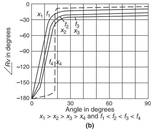
**Figure 2-4** Variation of  $|R_v|$  and  $\angle R_v$  with incident angle.
