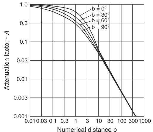
**Figure 2-11** Variation of attenuation factor  $A$  with numerical distance  $\rho$ .
