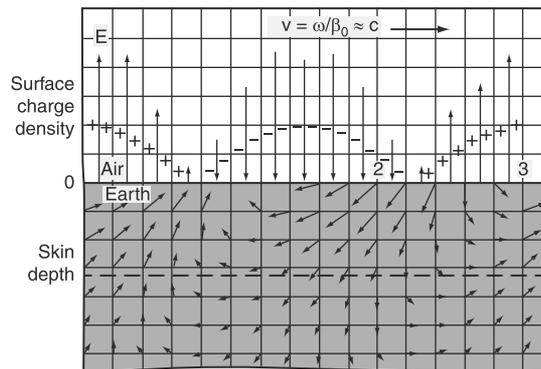
**Figure 2-8** Electric field, charge and current distribution.
