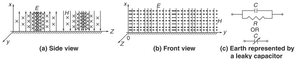
**Figure 2-1** Front and side view of the gliding wave and a leaky capacitor.
