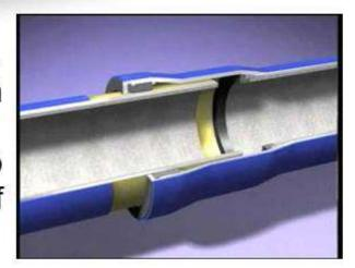
The spigot-end of one pipe enters the socket-end of the other. The joint is made by filling up the space between the two, partly by several turns of jute yarn and the remaining by pouring molten lead.
