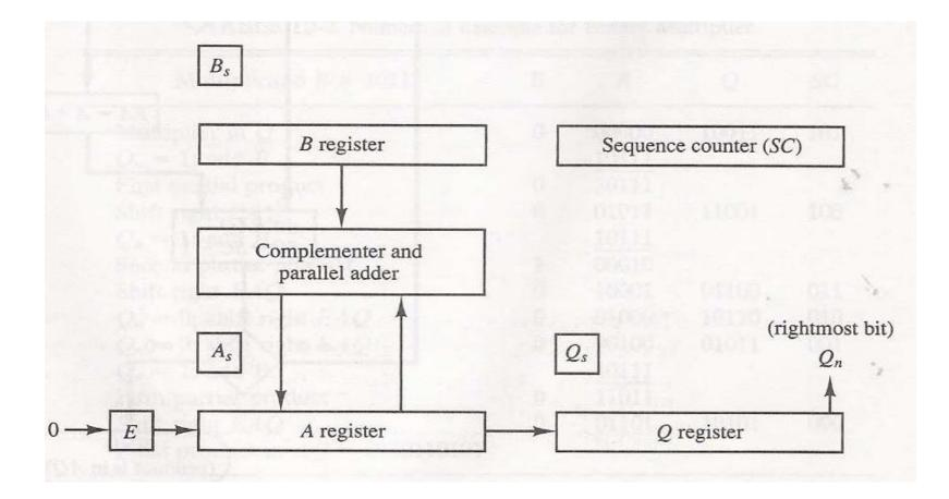
Initially, the multiplicand is in register B and the multiplier in Q. The sum of A and B forms a partial product which is transferred to the EA register. Both partial product and multiplier are shifted to the right.
