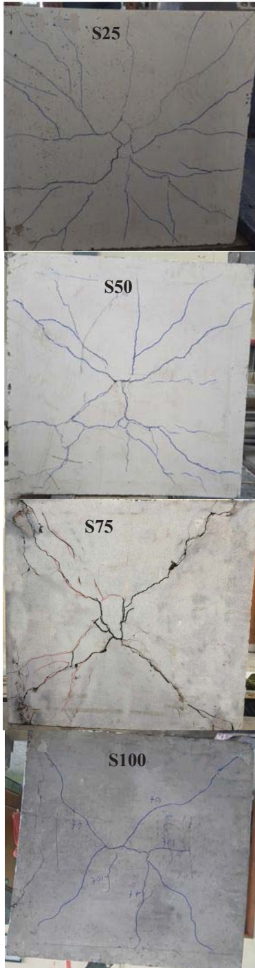
Fig.6. Mode of failure and crack pattern of slabs
