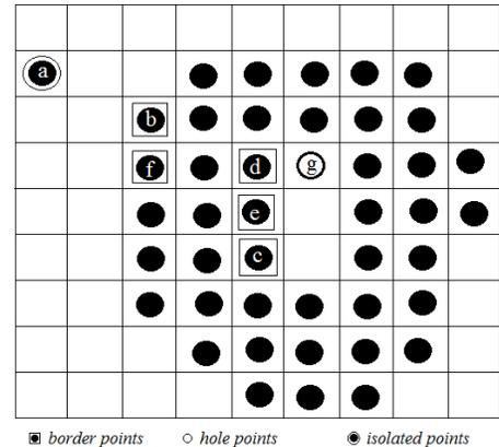
fig(3) Isolated, border and interior pixels
